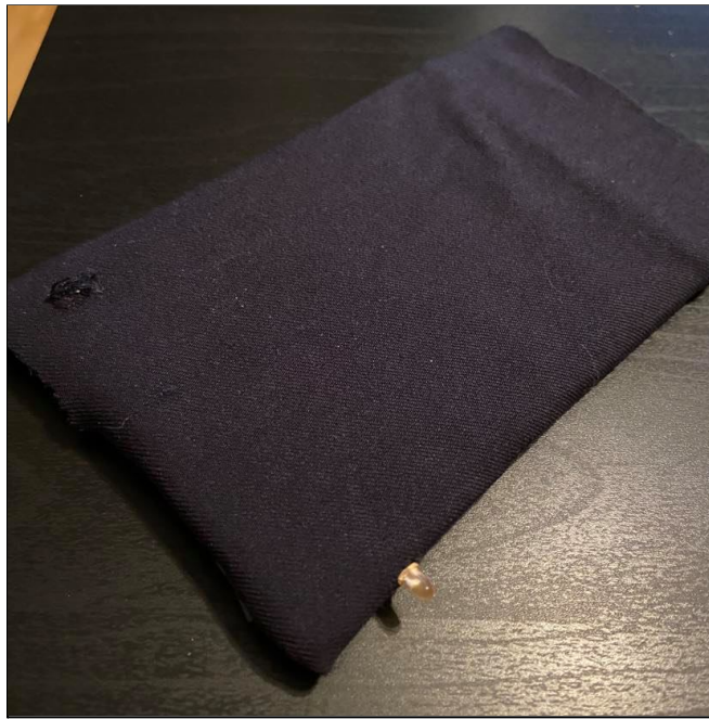
Figure 2. The model is made using a visually similar material. The lower left corner on the surface of the mat features a hole to be able to hold the temperature sensor. The lower right corner shows how the temperature sensor would be incorporated into the mat, sticking out of the side. This is shown with an LED.
