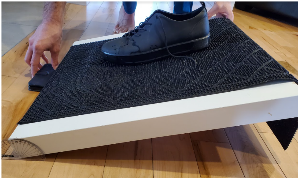
Figure 23. Grip test
