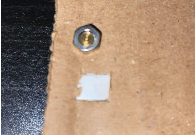
Figure 5. This view shows where the rain sensor will be implemented on the mat. A square surface would need to be cut from the material of the mat in order to properly integrate the sensor.
