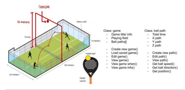
For our group design we decided to use a wide lens camera placed over the center line of the court. The combination of the wide lens camera and the elevation of the camera will allow the camera to see the entire court. Ideally, the camera would be placed 12 meters above the court and have 720p.
