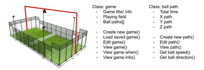
Max's design will feature one wide-lens camera centered above the court. As the game progresses the ball's position will be continuously logged in a text file along with the time. The stored positions are grouped each time the ball bounces off any surface.
