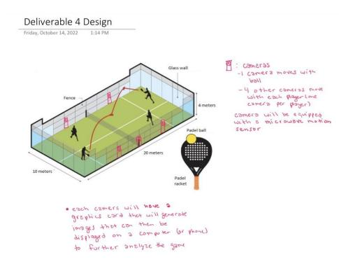
For Hannah's design, there will be 5 cameras installed on the padel ball court. There will be one camera for each person, which will move with them by tracing their movement. There will be two cameras on each of the longer sides of the court next to each player in order to trace their movement the best. There will also be a fifth camera placed on the side of the court, in line with the center line. The camera must also be higher than the net otherwise its view may be obstructed by the net.
