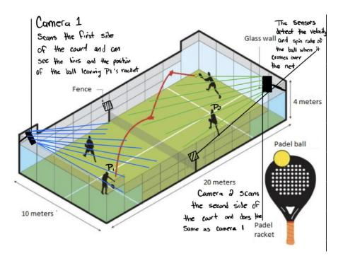
For Lucien's design, there will be 2 cameras placed in the corners of the court protected by pixy glass. Each camera will cover half of the court and get the location of the ball and the players, as well as where the racket is when the ball makes contact and leaves the racket.
