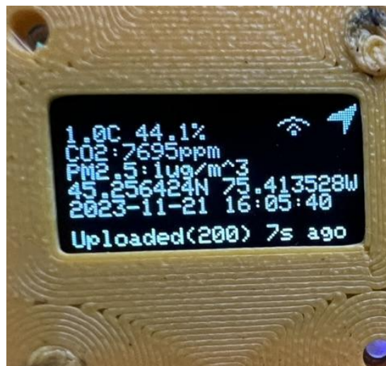
Fig 3: Device connected to Internet and GPS
