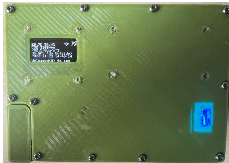
Fig 33: Device connected to the Internet but not GPS
