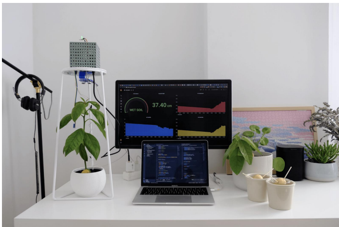
Figure 2: Example of Grafana display of plant growth data using Arduino sensors.
