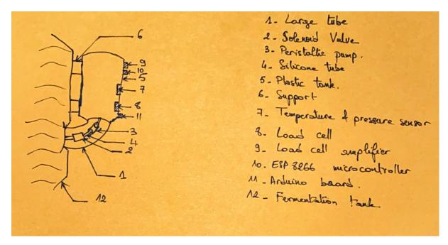
The improved device is a side tank that is attached to the main tank using adhesive blocks. The beer is transferred between tanks so the specific gravity can be calculated, then displayed using Loki Database and Grafana Cloud.
