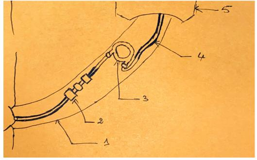
The two tanks are connected using silicone tubes. The transfer of beer happens thanks to a valve that opens and closes the tube and a pump that controls the flow of beer into and out of the side tank.
