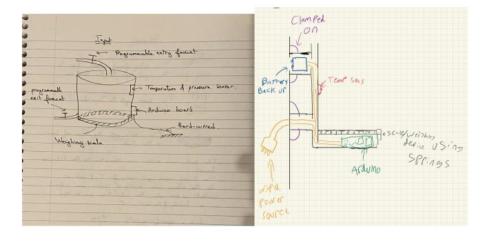
After our meeting with Shane, we decided to pursue Mohammed's sketch of the final design being a tank placed on the outside of the fermentation tank and connected with tubes along with Chris' design of the input systems.
