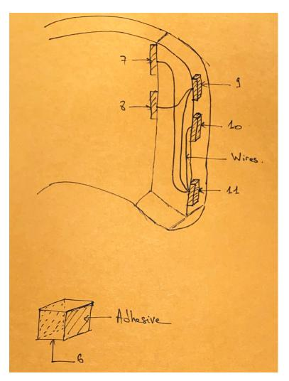
The temperature and pressure sensor as well as the load cell are mounted inside the side tank, which has a completely isolated hollow part on the side for easier wiring. The temperature and pressure sensor is directly connected to the Arduino board, whereas the load cell is connected to the load cell amplifier first, which increases the accuracy of the mass values that are later sent to the Arduino board. We are also using an ESP8266 Microcontroller to connect the device to WiFi.
