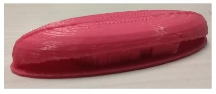
along its minor axis. Therefore the model is at a 1:731 scale. The model was created in Blender, and then 3D printed at the Richard L'Abbé MakerSpace. As part of the printing process, there were structural supports under the various overhangs caused by the roof, however those were removed prior to the tests.
