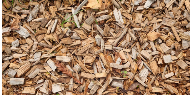
Figure 9: Example of wood chip layer (WCL) for use as insulating layer for snow pile.
