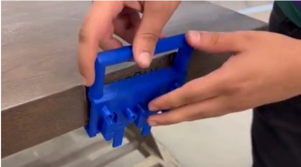
Video 1 Jig being clamped on a door. You can find the video here .
