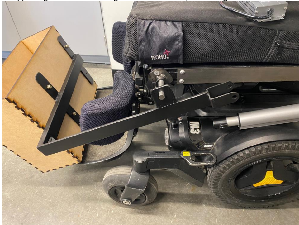
Figure 3.12 Removing rotating assembly and linear actuator linkage.
