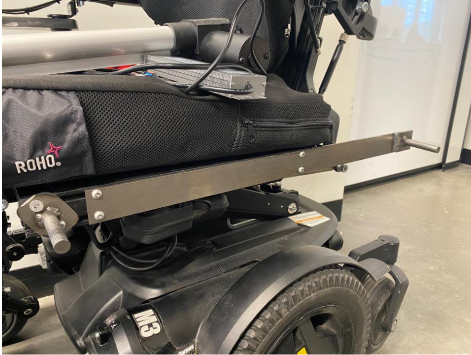
Figure 3.5 Completed mount installation.
