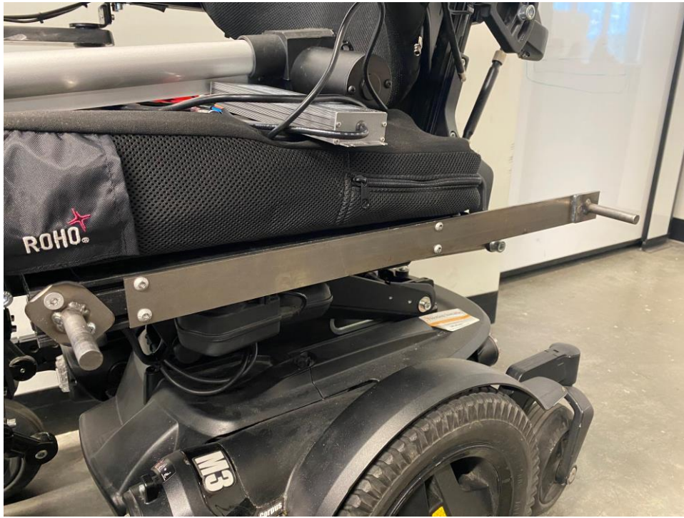
Figure 3.13 Removing mounting hardware.
