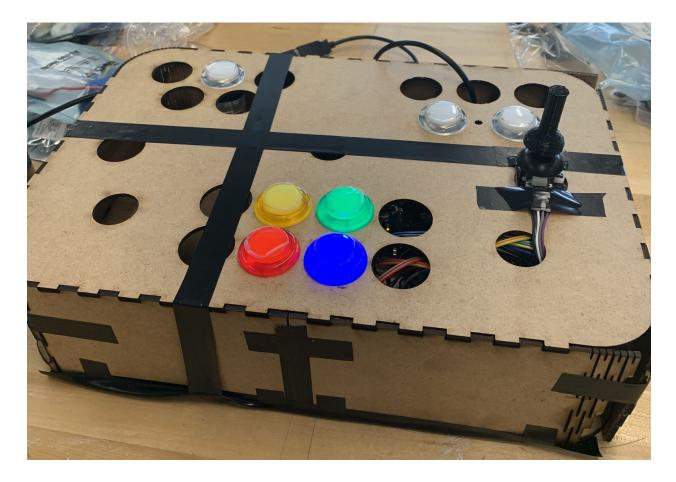
It includes 7 arcade buttons, that are fitted to the top of the case, a controller case, and the joystick covers attached to 1 joystick.
