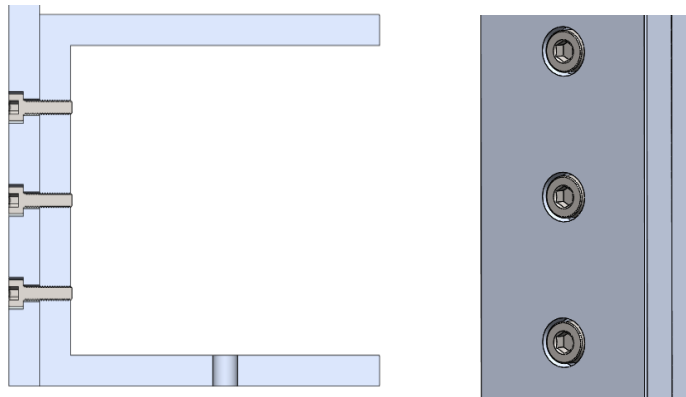
Figure 17. Flat Bar Screwed to C-Channel
