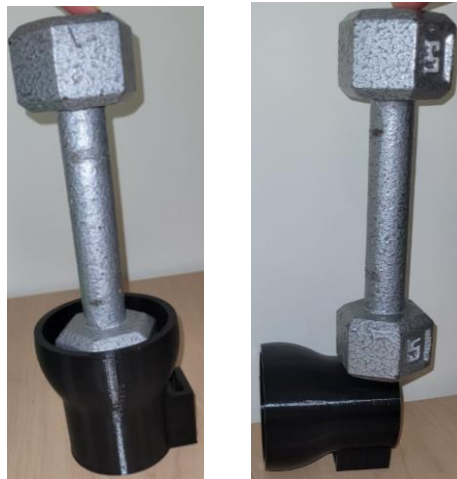
Figure 22. Longitudinal Compression Test (Left), Diametral Compression Test (Right)
