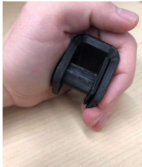
Figure 26 - Plunger of P1 Test 2 compressed
