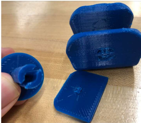
Figure 31 - P2 Test 2 Point of failure
