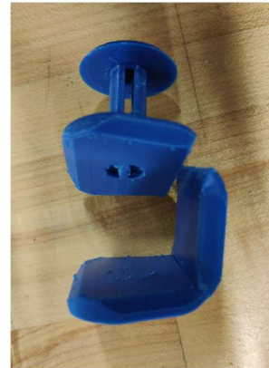
Figure 32 - P2 Test 2 Point of failure on body
