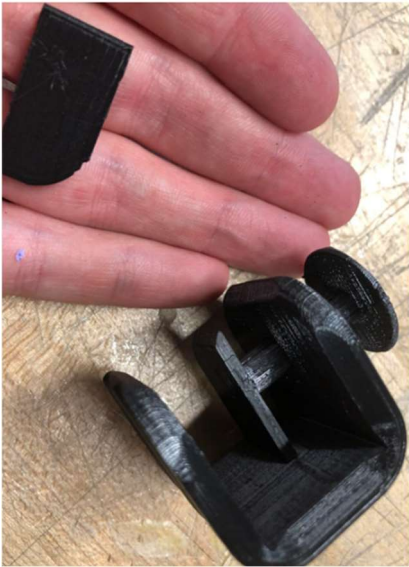
Figure 33 - Damaged compression plate
