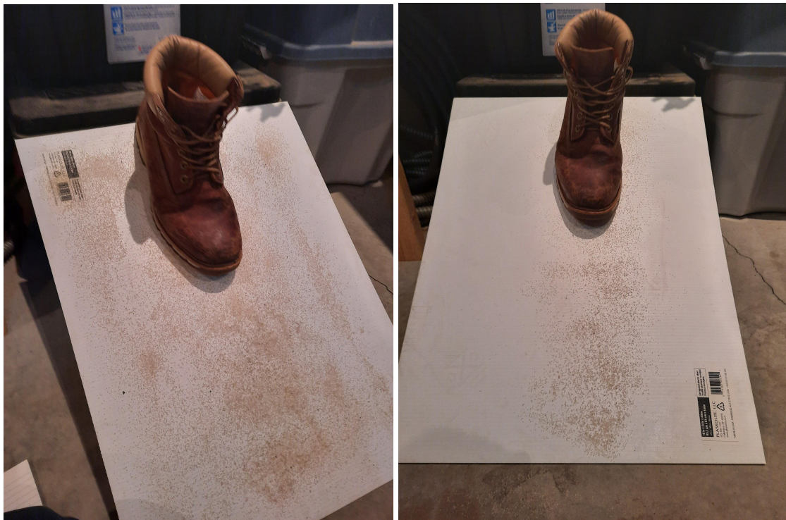
Figure 2 - Boot on Grit stopped by Static Friction (2 layers left, 1 layer right)
