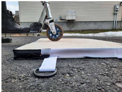
Figure 14 - Wheelchair Accessibility Test with Scooter
