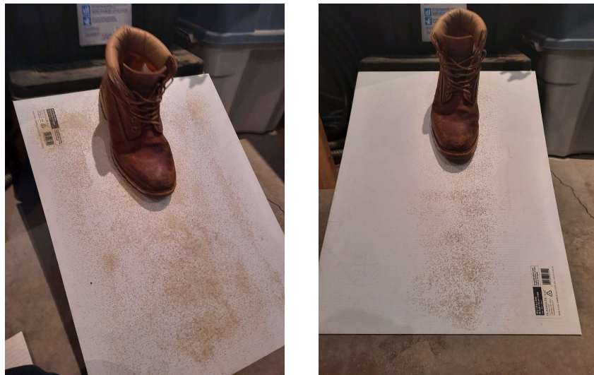
Figure 9 - Boot on Grit Stopped by Static Friction (2 layer of grit on left, 1 layer of grit on right)
