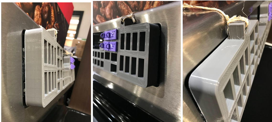
Figure 6: Images above showing how the grid is dimensioned so it sits flush to the control panel set into the backboard.
