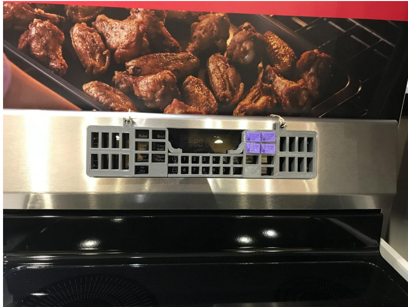
Figure 4: Wide view of the grid sitting on the control panel, all buttons are covered and sequestered in the slots.
