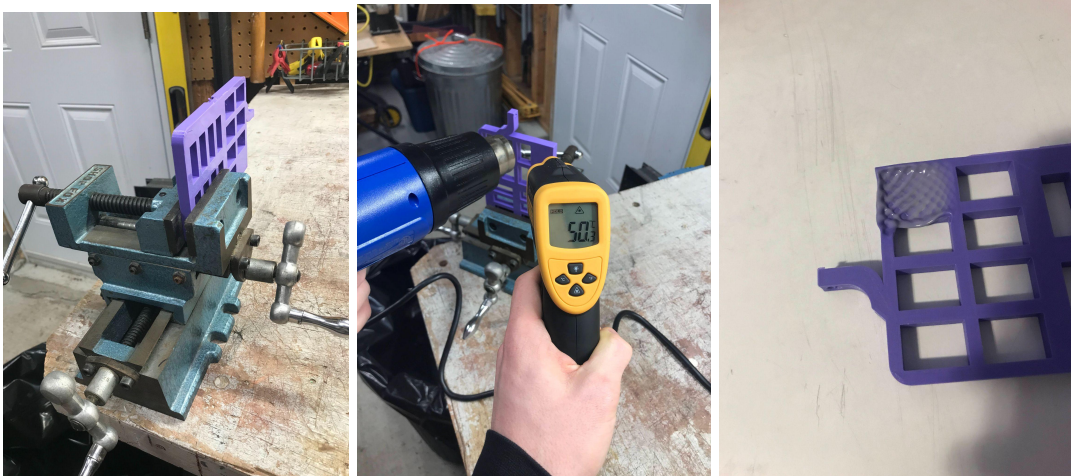
Figure 3: Failed print held in the vise clamp (left), heat gun and temperature monitor used to perform the PLA heat test (centre), resultant deformation of the grid (right)
