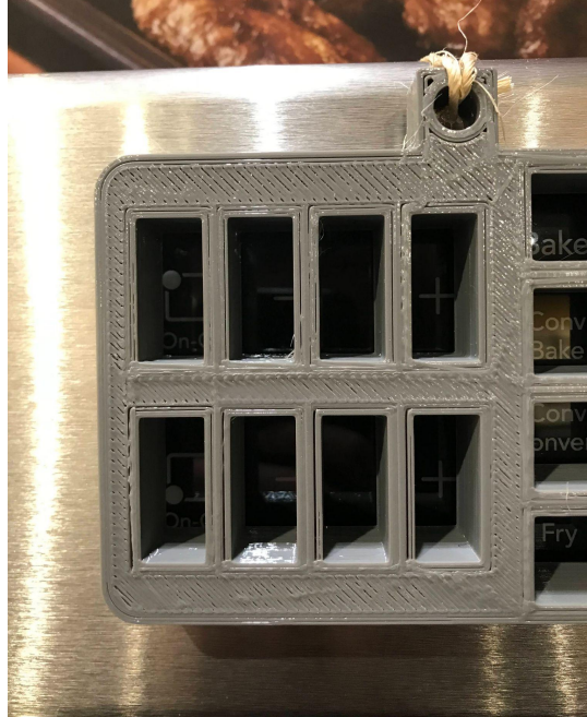
Figure 8: Misalignment of dimensions with the outer eight buttons (4 top and 4 bottom), this problem is repeated for the right side.
