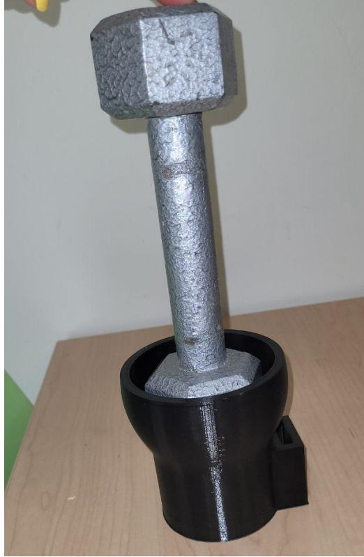
Figure 5. Strength Test Longitudinal Compression
