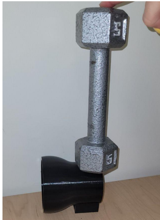
Figure 4. Strength Test Diametral Compression
