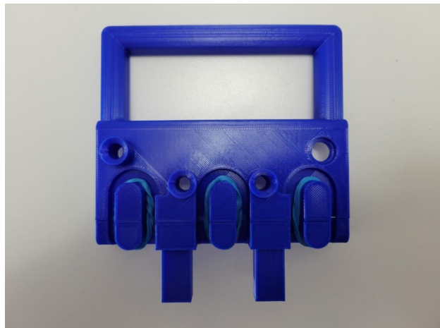
Figure 2 Rubber bands used for the sliding part
