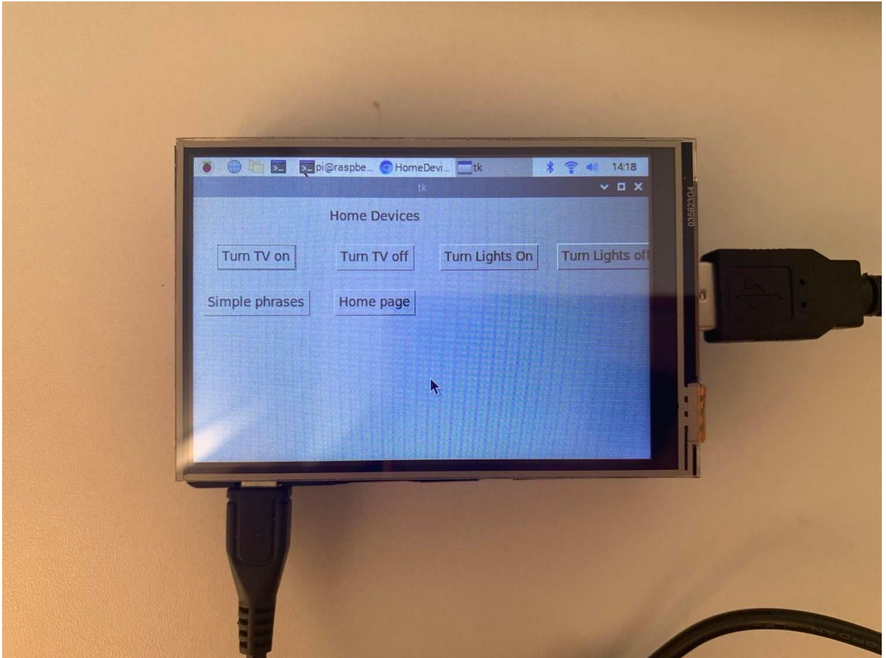
Figure 6: “Home Devices” phrases displayed as buttons, ready to be voiced via speaker
