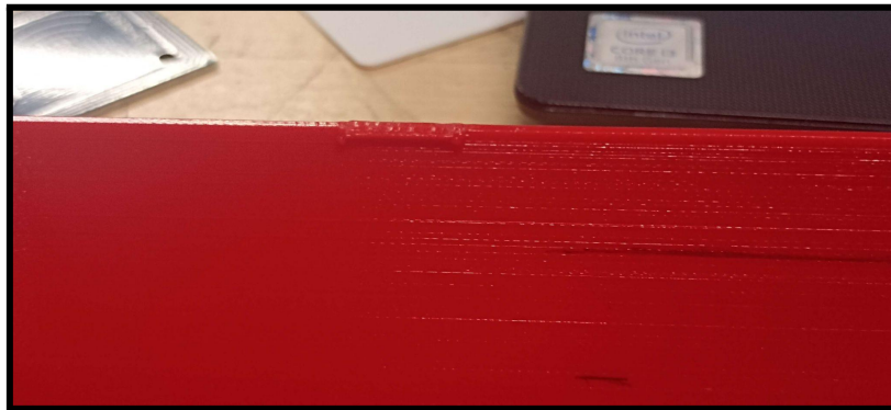
Picture of one of the casing's two attachment points (a small extrusion of 1.2 cm in length and 0.5 mm in depth)
