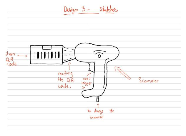
This barcode scanner reads and decodes information encoded in a barcode. It uses a light source and a sensor to capture the patterns of dark and light bars in the barcode, converting them into a digital signal. This data is then processed and can be used to retrieve product information, track inventory, entries and exits of an item, or perform various tasks, such as pricing, in a fast and accurate manner.
