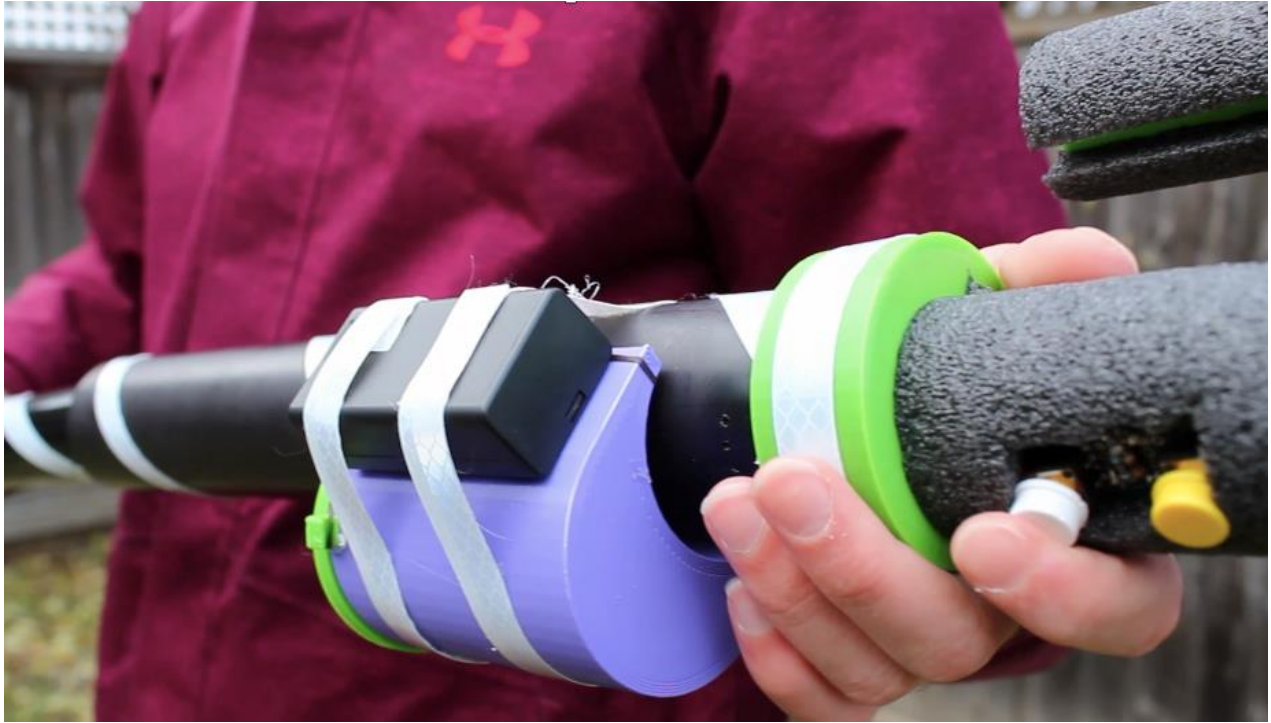
Figure 5: Buttons and electrical components on the permanent handle of the cane.
