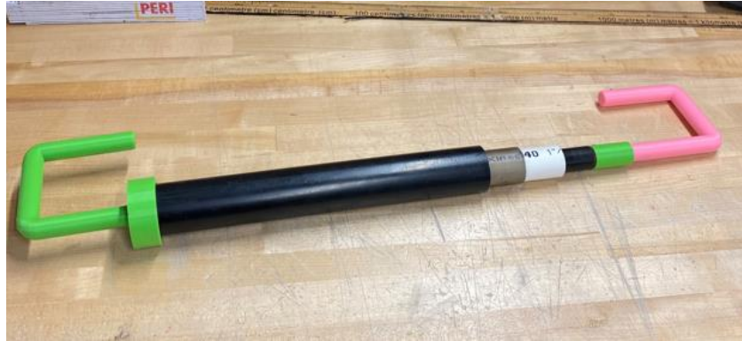
Figure 12: Installed 3D Printed Handles
