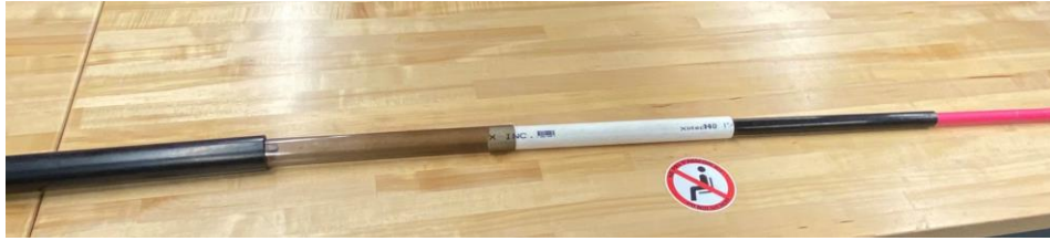
Figure 10: 4 PVC Pipes Installed with 1 3D printed Segment
