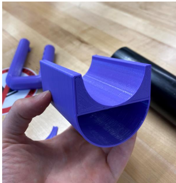
Figure 11: 3D Printed Navigation Compartment
