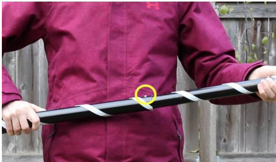
Figure 3: The spring pin peeking through the hole in the segment.
