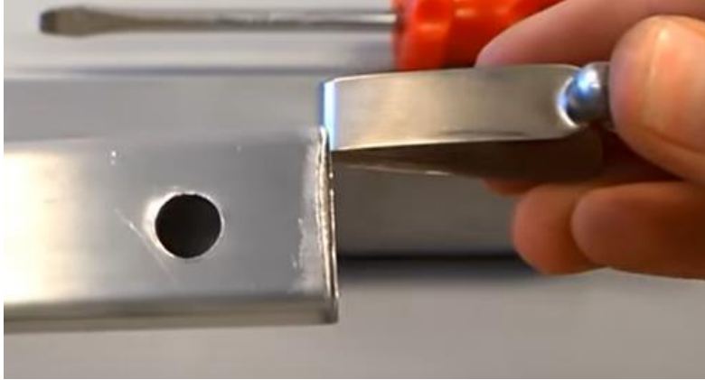
Figure 8: Demonstration of the Push Pin being Inserted into a Pipe Segment [2]
