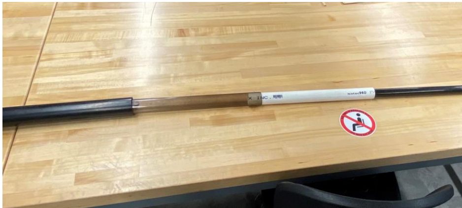
Figure 9: Four PVC Pipe Segments Assembled with Spring Pins
