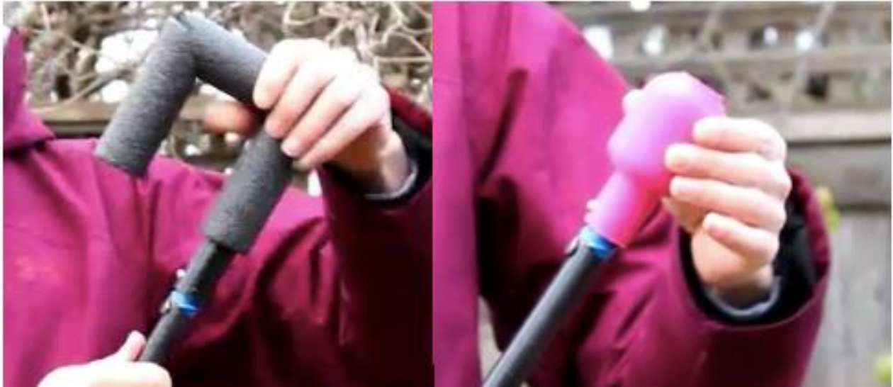
Figure 4: Both handle options locked in place, by spring pins.
