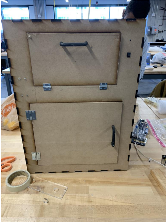
Figure 5: Image of the Attached Doors and Handles by Hinges and Screws
