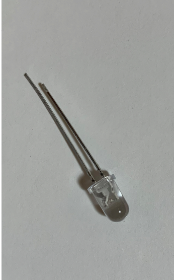
Figure 15: Image of the LED Light showing the Negative Short Leg
