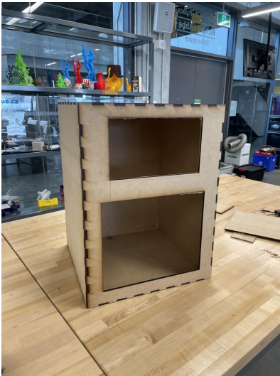
Figure 1: Proper Configuration of MDF Board Frame
