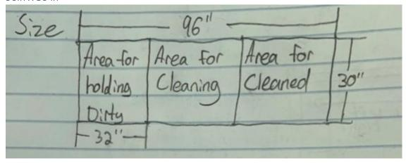
This design shows which areas the boards will be in during all the processes of being cleaned. It all fits within the size constraints in our specifications. It could be more compact but otherwise meets our needs for a table design.
