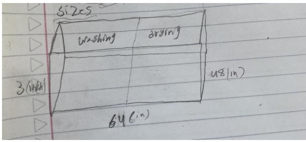
The height of this cleaner is 3 inches, the length is 68 inches, and the width is 48 inches. Half of its size cleans rafts and the other half dries rafts. The disadvantage of its size is that it can clean 1 raft each time and dry 1 raft each time. Is not capable of cleaning lots of rafts for busy days.
