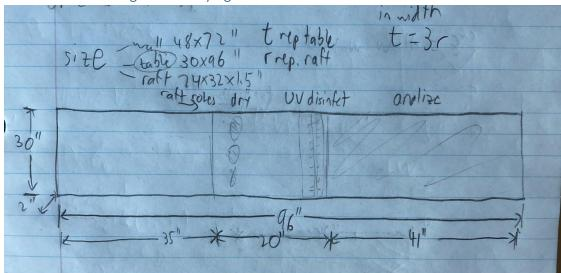
This cleaning system fits on the table. Its expected size is 30x55 inches and the table is 30x96 inches. This leaves 41 inches of space to take the board from the machine/analyze it.
