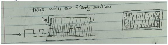
This concept only uses a hose with some eco-friendly sanitizer to kill the algae and a bunch of brushes. The raft gets pushed through the device which has brushes that cover the whole machine. It should be good at cleaning the tops and bottom of the raft. A large downside is that this will either be very hard to replace, which doesn't align with our specifications, or it won't last long because it relies on all the brushes to last long and work long.
