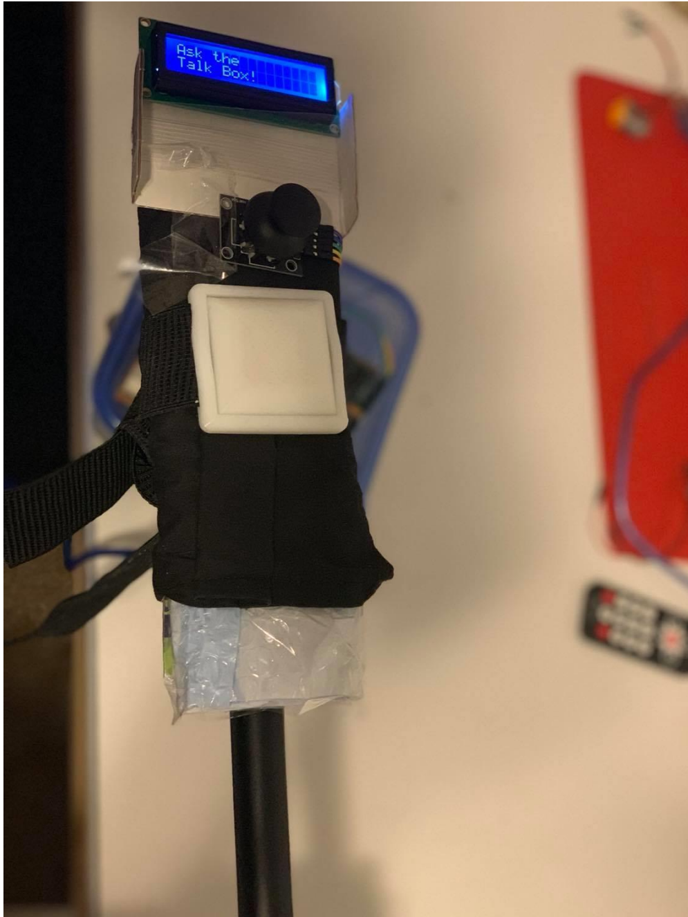
Figure 5: Prototype of the wheelchair tubing frame and armrest with talk box joystick and button
