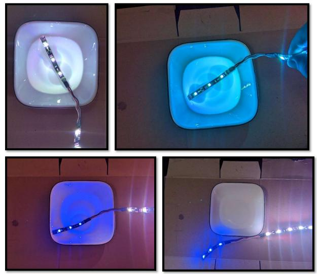
After submerging the LED strip and the recently soldered connections, the lights still function.
