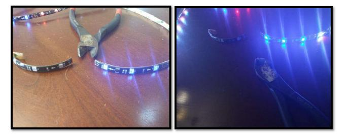
After cutting the lights, the remainder of the strip still functions properly with all the integrated features.
