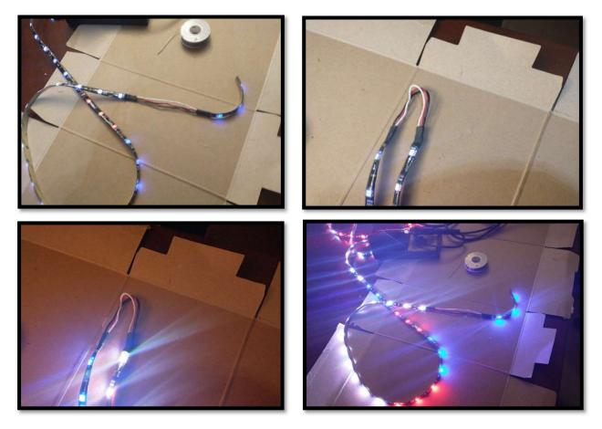
After a little struggle with learning how to solder properly, the lights were reconnected and still functioned properly. As demonstrated in the picture above, the connections still work, and we added heat shrink to solidify the connections and to waterproof it.
