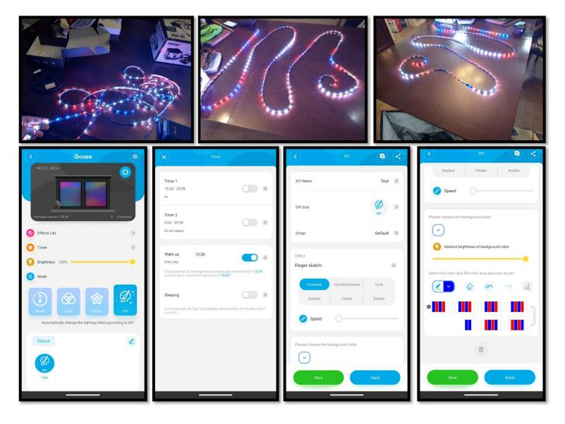
Once plugged in, the LED lights immediately turned on an emitted bright light. After downloading the Govee application and connecting to a Bluetooth connection, the LED strip was easily controllable from a smartphone. This allowed us to segment different parts of the light. Also, the application allowed for wake-up and nighttime timers which allowed us to program an artificial sunrise and sunset.
