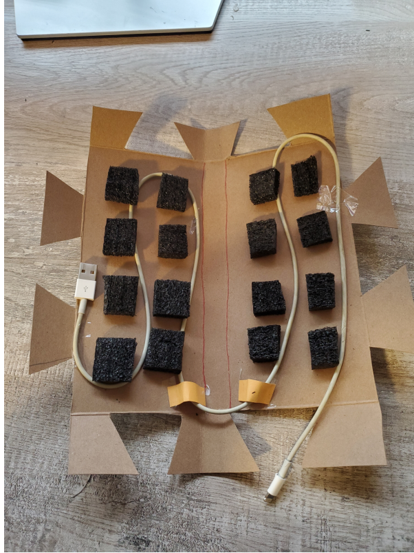
Figure 1. Cardboard prototype of the mat and internal structure
