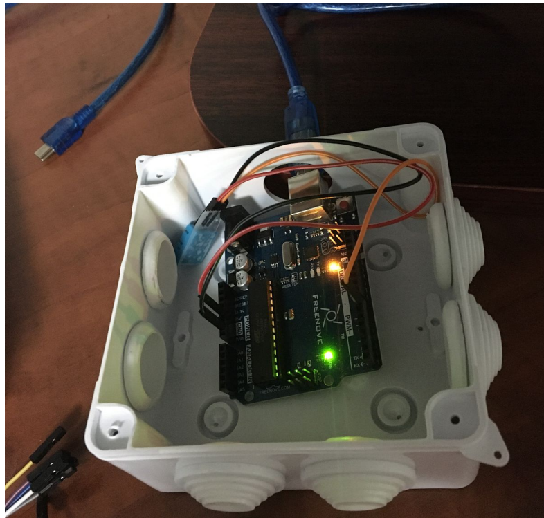
Figure 2.1 - Arduino Uno inside the housing for the heating test
