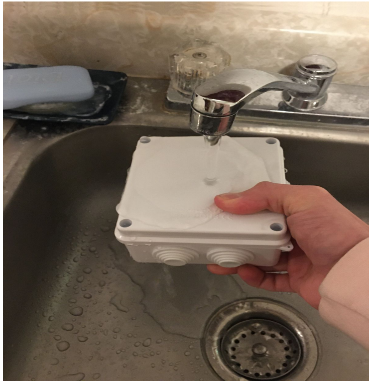
Figure 3.2 - Housing waterproof test
