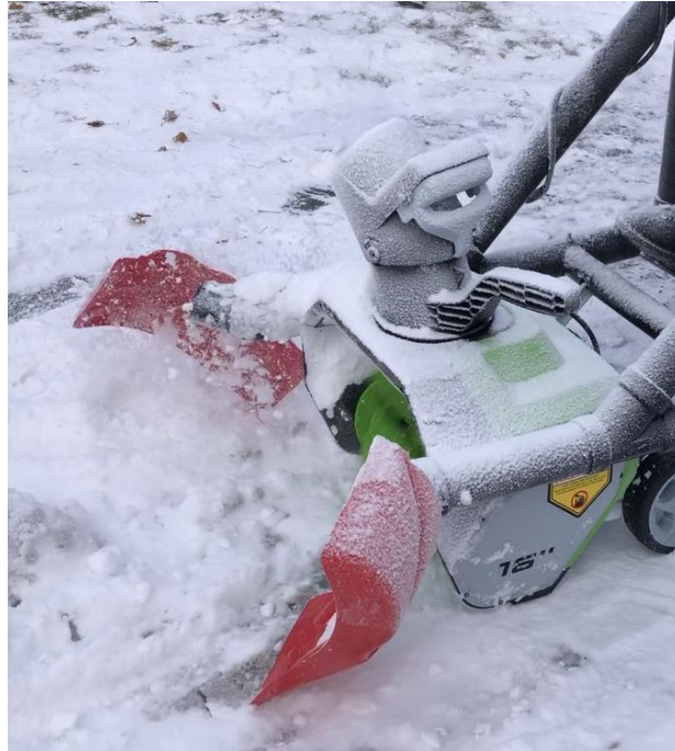
Figure 5 - Moment of Failure of Shovel Guide
