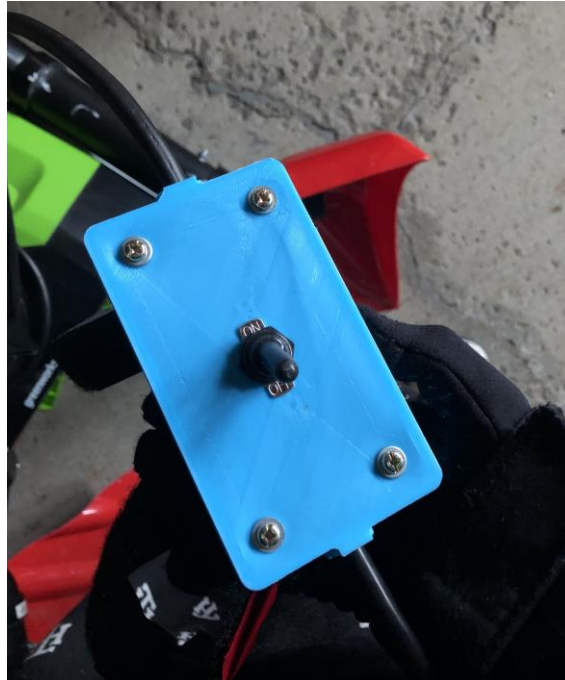
Figure 3 - Electrical Switch Box
