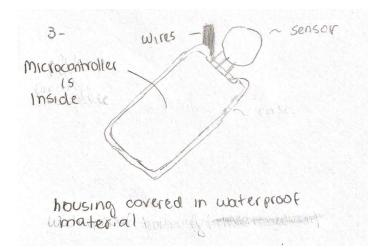
Waterproof cover made for the housing, preventing contact of the microcontroller with water
