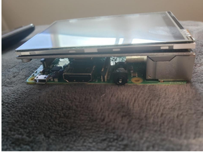
Figure 6.4.1.3 Mounting the screen
