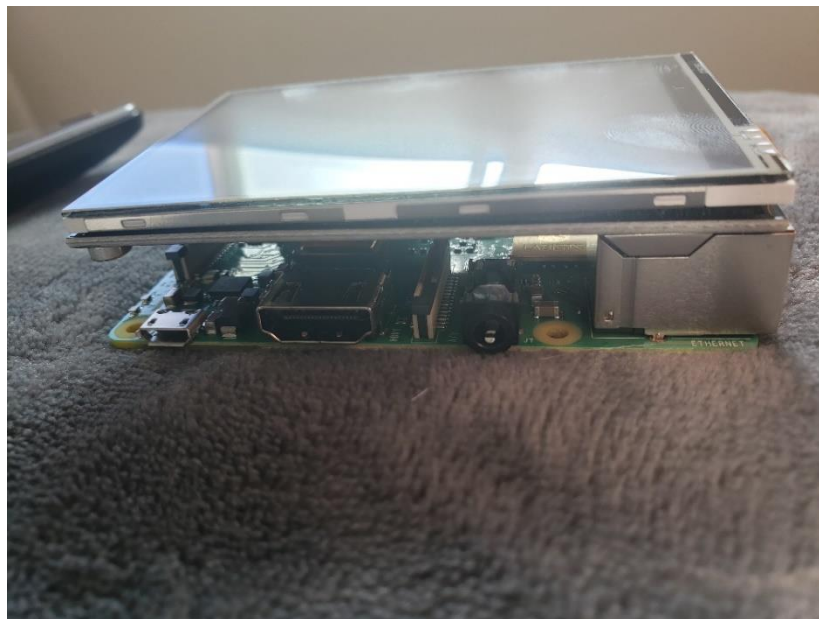
Figure 6.4.2.1 Mounting the screen
