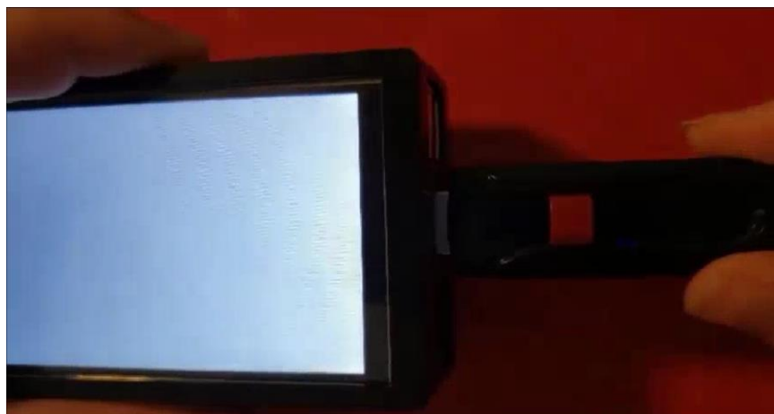
Figure 3.1-2 Plug USB Stick into the Side of the TalkBox
