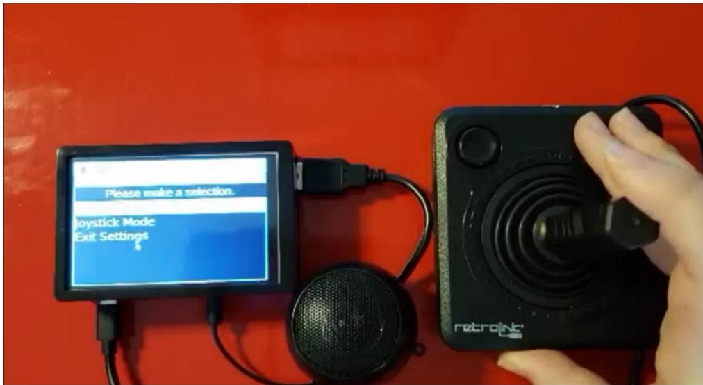
Figure 3.1-1 Speaker Connection, Joystick Connection and Power Connection
