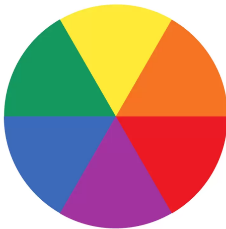
Figure 25 - Colour Wheel Blue: Temperature out-of-range Red: Violent shake Yellow: Humidity out-of-range Green: Temperature and humidity out-of-range Purple: Violent shake and out-of-range temperature Orange: Violent shake and out-of-range humidity White: Violent shake, out-of-range temperature and humidity
