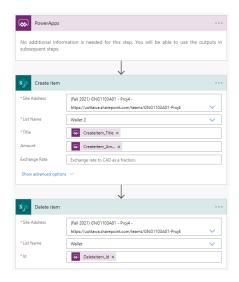
For the transfer of points between SharePoint list databases, a flow was created that deletes and item from one list and adds it to another. This flow was then added to PowerApps, so when a button is pressed the flow runs.
