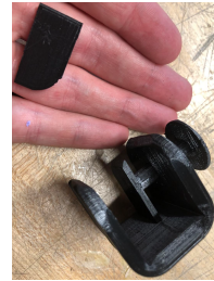
Trial 2: Weak Compression Plate
