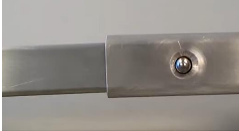
Figure 14: Demonstration of the Locked Spring Pin Mechanism [1]
