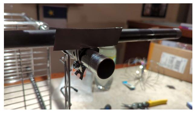
We have cut and shaped 2 small pieces of rectangle sheet metal and attached it onto the handles of the walker. The steel bar that contains the brakes would just slide right in between them.
