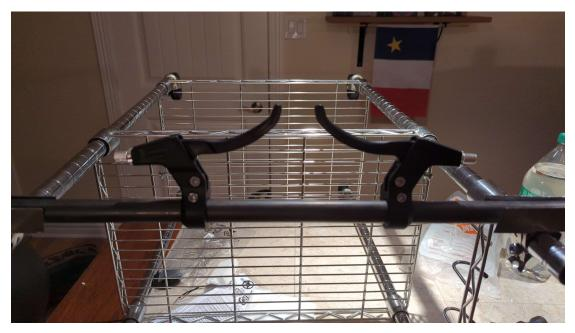
Brakes are attached in parallel to the bar. Once you press the right brake the brake on the right hand side will get triggered and vice versa for the left side.
