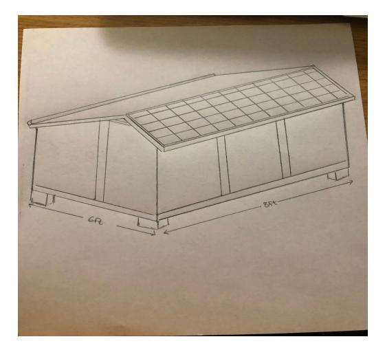
This idea was to design a greenhouse that would maximize light absorption and be able to collect rainwater . The solar panel would be placed on the top end to achieve as much power as possible and the on the other top end would be a slope that would be able to collect rainwater. The figure of the greenhouse will be a rectangle figure with 8x6 feet dimensions. This design was decided on to keep an effective and simple design.
