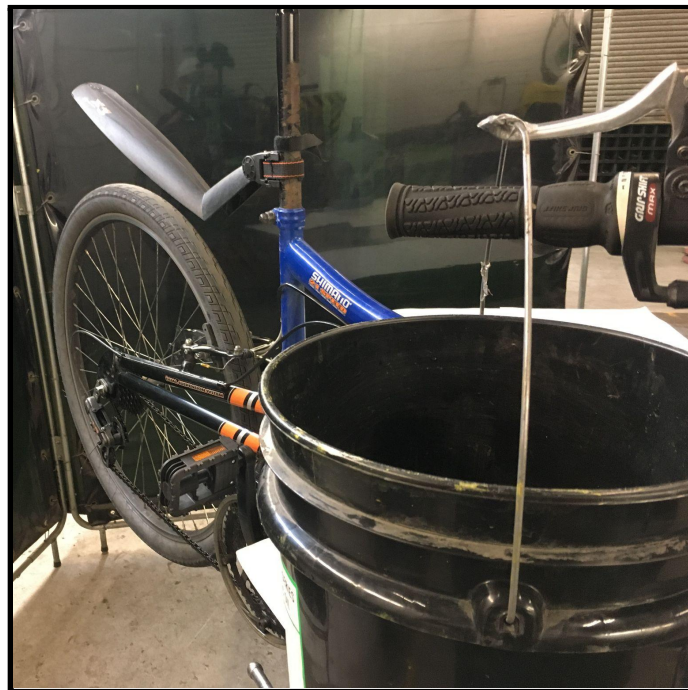
Figure 37 - Force test using a bucket filled with water to measure the braking force
