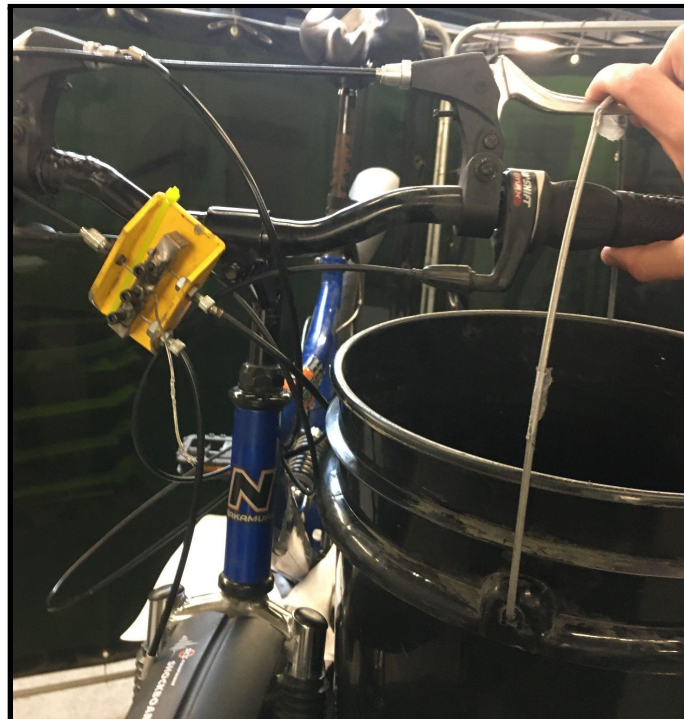
Figure 39 - Force test using the cable splitter
