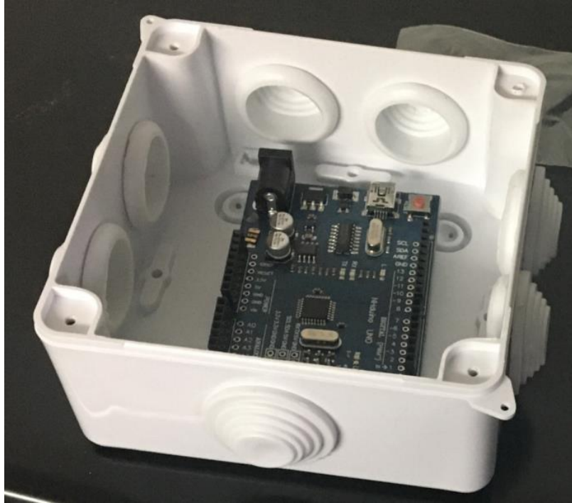
Figure 4.5 Arduino in Junction box
