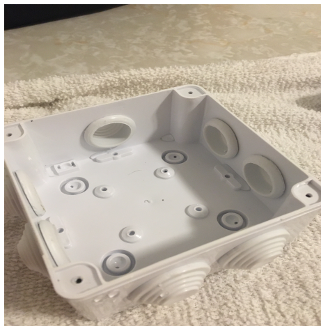
Figure 6.14 Inside of the housing was not affected by the water.
