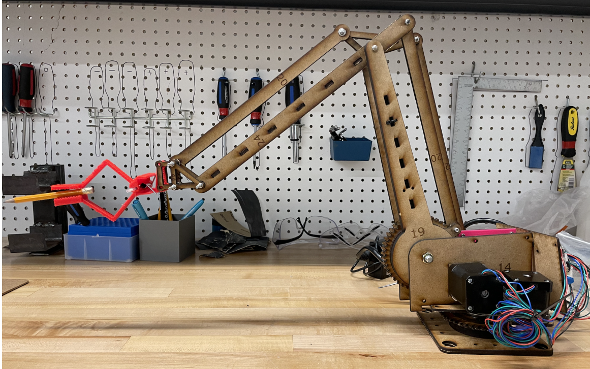
Figure 15. The end-effector holding a paintbrush while being attached to the arm. The purpose of this test was to determine if the arm had the structural strength to hold the combined masses of the end effector and another object.
