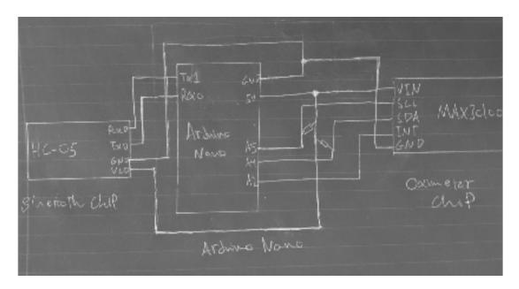
An outlining diagram for the connection of essential device components has been created (the boxy connections are 4.7k ohm resistors). We can begin the construction of the prototyping circuit once the components are here.
