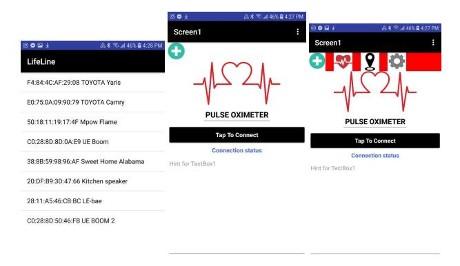
Showcasing the current state of our application: The pulse oximeter screen has the option to connect to bluetooth to a chosen bluetooth device, shows if the application is connected, and has a working toggle menu.
