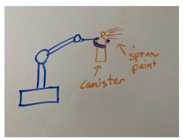
This end-effector design uses a canister of spray paint. This design is simpler than a nozzle, but more wasteful.
