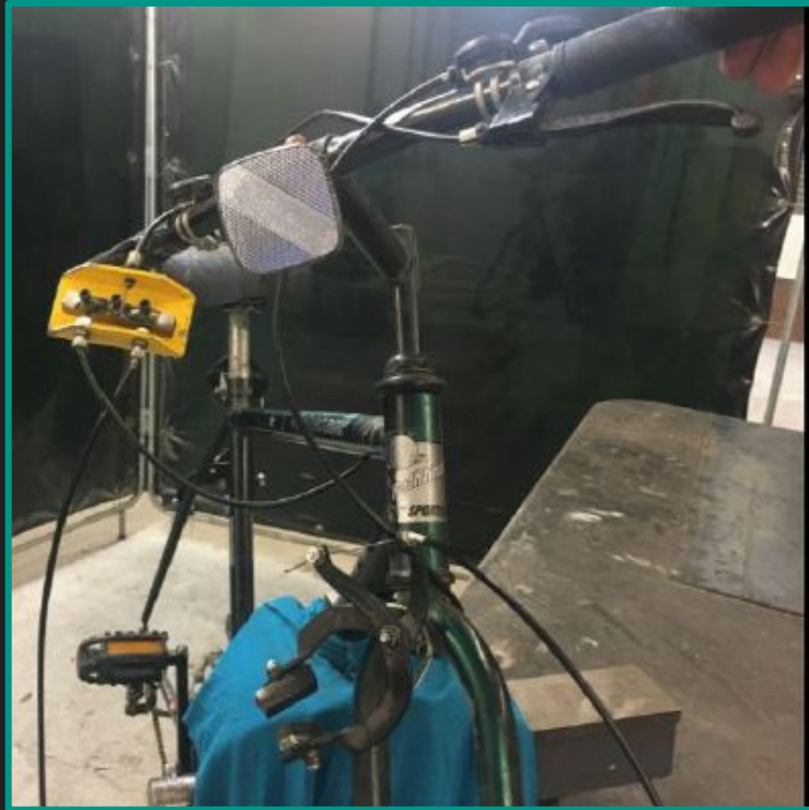
Cable Splitter on Bicycle
