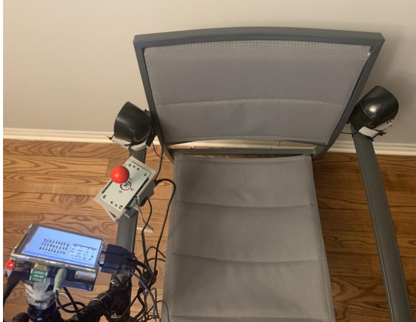
Figure 2-2: Gooseneck with user screen, joystick and speakers mounted on chair
