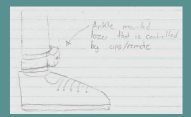
This is a laser mounted on a ankle band which emits laser pointers on the ground. This is proven to be a walking stimulus since this would motivate the patient to walk over the laser pointer every time the walk.
