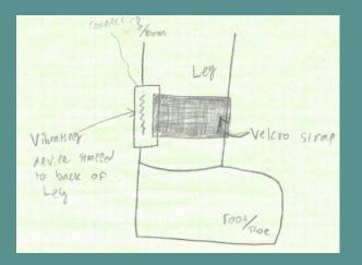
This is device that is also mounted on the ankle but except there is a vibrating device attached to it that stimulates the ankles resulting in the patient walking. The device is attached on a velcro strap so that it is convenient for the patient to put it on and off.
