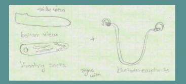
This a vibrating sock that is sync with bluetooth earphones. The objective of this design was to stimulate the patient to walk by vibrating their feet. As they take a step their foot starts vibrating for 5 seconds and at that exact moment a beat is produced in the earphones. This design was based on the fact that audio stimulus is another working device that could motivate the patient to walk.
