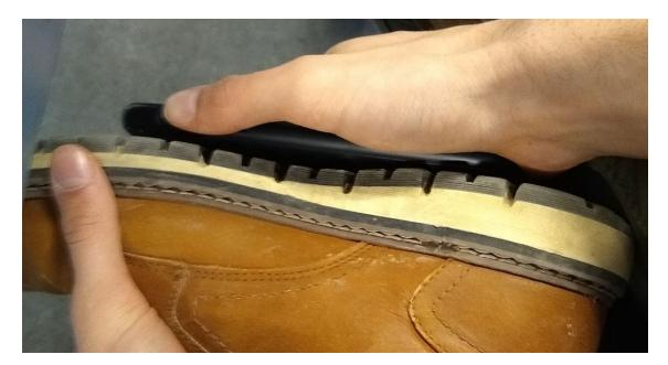
While a phone vibrating motor is not a perfect analogue to the motors which will be used in the final product, this test demonstrates that even small amounts of vibration can be felt through a thick shoe. The motors selected for use in future prototypes are stronger than a phones vibrating motors, and there will be more of them working to send vibrations through much less material.
