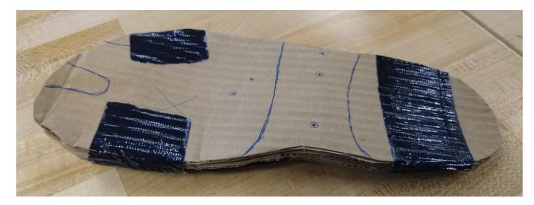
The test was determined to be a success, as the placement of the glass gems did not prove uncomfortable. Additionally, the additional layers of cardboard slowly adjusted to better fit the shape of the foot and shoe. Unfortunately, the cardboard insole was thicker towards the toes, and it made for some discomfort, but since there were no motors or wires in the toes, that can be easily shaped for a better fit in future prototypes.
