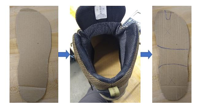
After the areas of highest load were determined (The areas marked with a faint X in the rightmost picture), The placement of three sample motors was determined, and templates of the insole were constructed with extra cardboard. Holes were then cut into the extra cardboard to allow the placement of the small glass gems which, while not a perfect analogue for the vibrating motors given their rounded tops, will serve as adequate material for initial testing.
