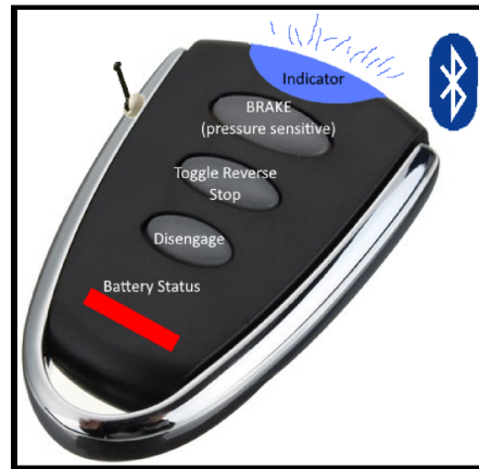
Figure 7 - Rough design of the controller with updated button functionalities
