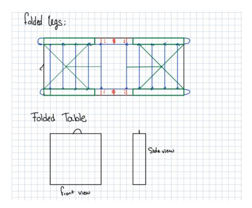
The rod in the middle will shrink allowing the legs to fold in and lock in place, the hinges will then unlock allowing the table to fold in half and the small hook on the side will hold the table in its closed position.
