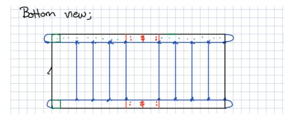
Metal rods soldered to the Rods on the side in order to hold the mesh in tension , while reducing the sinking effect to its maximum and providing back support.
