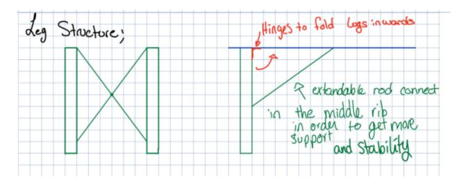
X-structure for stability. This will be achieved with aluminum rods that will be soldered to the corner of the legs.
