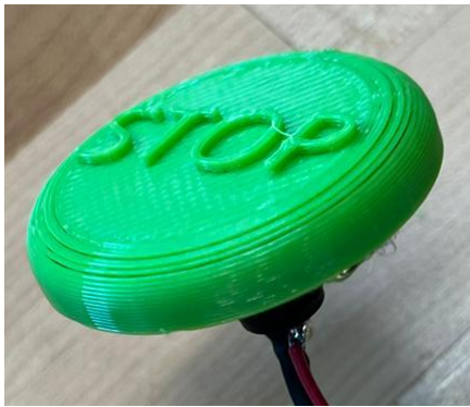
Figure 10: Emergency Stop button labeled "STOP"
