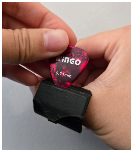
Figure 4: Inserting the guitar pick into the back of the slot
