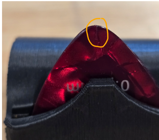
Figure 46: Notch cut into pick to measure horizontal displacement
