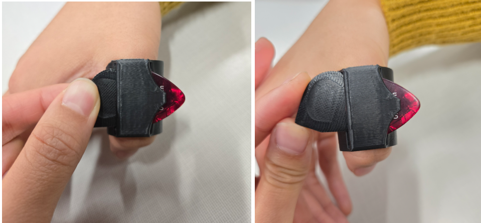
Figure 10: Pull the wedge from the slot (left), or rotate the wedge from the slot (right)
