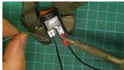
Figure 28. Solder the wires to the Toggle Switch
