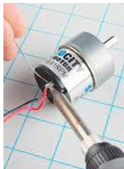
Figure 26. Solder the wires to the motors
