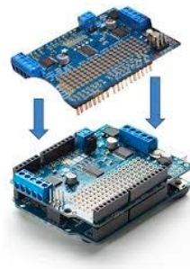
Figure 22. Connecting the motor shield to the Arduino
