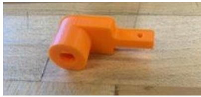
Figure 4. 3D Printed Motor Attachment and Flap
