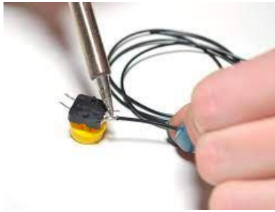
Figure 27. Solder the wires to the Push Button
